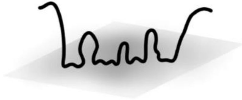
Fig. 1. Flexible, unordered polymer molecule adsorbed at a surface
